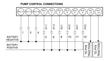
Section 5.4.4 Typical Brush Wear Sensor Connections For Pump Control
