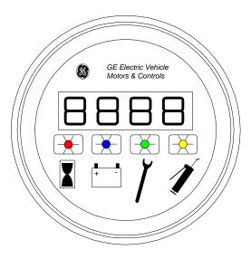
The GE Standard Dash Display is a four segment Light Emitting Diode (LED) instrument that displays the GE LX, ZX, and SX Status Codes, Hourmeter Readings, Battery Discharge Indication, and Maintenance Required Code. The four LED's above the symbols indicate the active readout mode.
